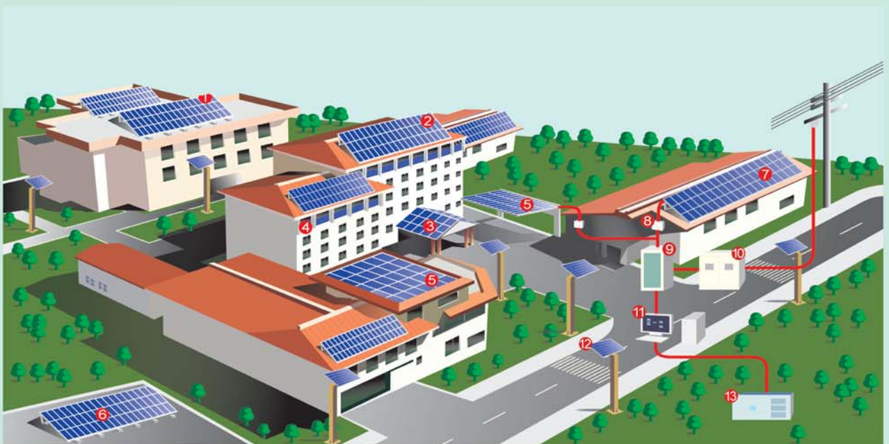
⑦ Solar panel ⑧ Terminal box ⑨ Inverter ⑩ Distribution device ⑪ Monitor ⑫ Road lamp ⑬ Display
